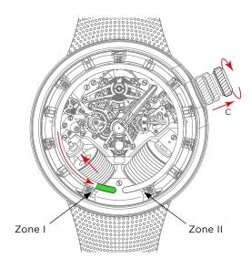
**Important:** If you plan to not wear the watch for a while, the colored liquid has to be stored in its own reservoir (on the left bellow).
