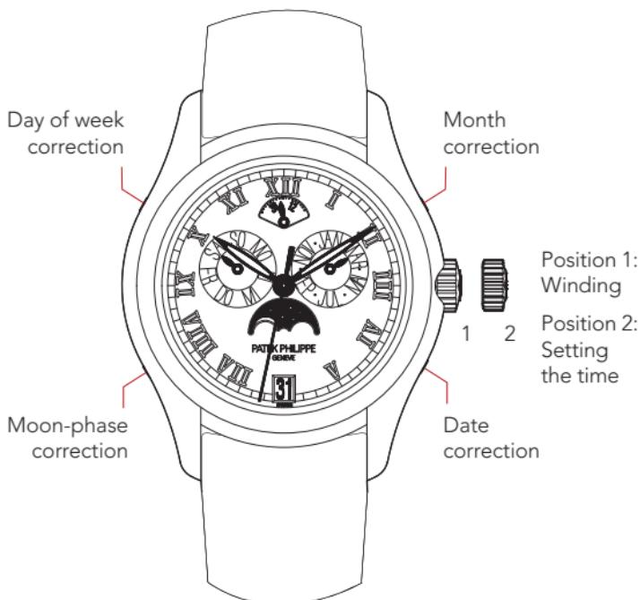
The diagram applies to all self-winding watches with Annual Calendars and caliber 324 S QA L or 324 S IRM QA LU movements.
