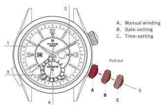
Ø 42 mm, TUDOR calibre 2892 with additional mechanism for the alarm function, waterproof to 100 metres (330 ft). Date (pointer-type display), alarm power reserve.
