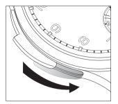
The repeating slide is operated as shown in the illustration. You must always fully depress the slide; otherwise, the repeater will not be activated. This "allor-nothing" principle ensures that the watch does not chime the time incorrectly. You can then allow the slide to return to its original position.
