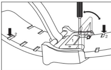
opened simply by inserting the special tool supplied with the watch into one of the two bore holes and lifting the locking lever. After opening, the locking lever should form
