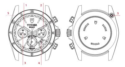
Ø 42 mm, TUDOR calibre 7753, waterproof to 150 metres (500 feet). 12-hour chronograph, date (date window), small seconds hand, black-lacquered steel bezel, crown guard, bistable pushers.
