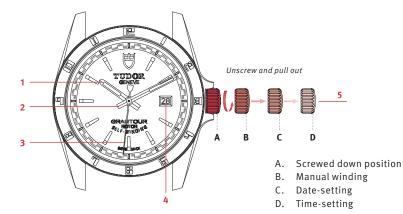
Ø 42 mm, TUDOR calibre 2824, waterproof to 150 metres (500 feet). Date (date window), black-lacquered steel bezel, crown guard.
