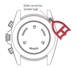
It is essential not to adjust the date between 20:30 and 23:00, to avoid damaging the movement.
